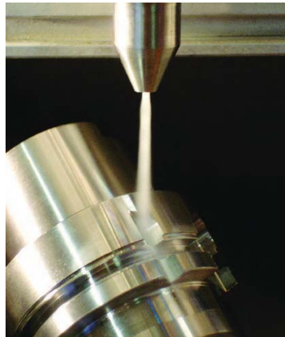
The CO 2 snow-jet technique offers significant time and money saving potentials for cleaning functional areas such as sealing, joining and bonding surfaces.
