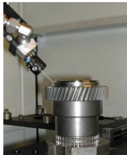
To ensure that parts are sufficiently clean for the subsequent laser welding process, welding surfaces are cleaned with CO 2 in-line beforehand.
